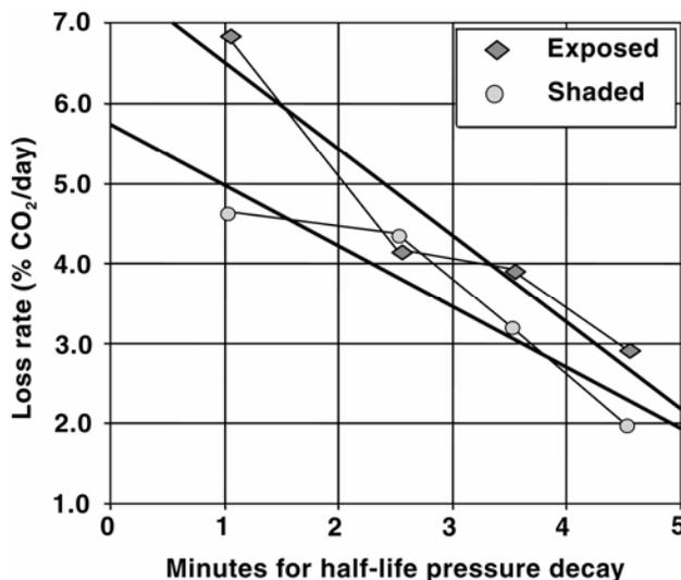
Fig. 18. Loss rate of carbon dioxide from a treated empty structure of 7.5-m<sup>3</sup> capacity in relation to half-life pressure-decay time. The suggested maximum loss rate is 2% CO<sub>2</sub> per day. (Data from Navarro and Zettler, 2001)
