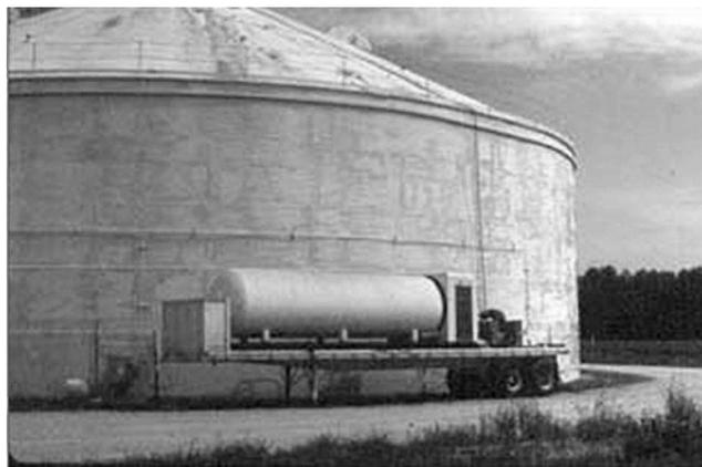
Fig. 1. Application of carbon-dioxide-based modified atmosphere in a large silo bin in Kingston, NC, U.S.A.
