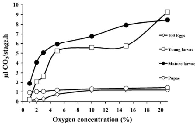
Fig. 9. Respiration rates of the development stages of *Tribolium castaneum* at different O<sub>2</sub> concentrations in nitrogen at 30°C and 70% RH. (Adapted from Emekci et al, 2002)
